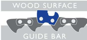
The cut clearance causes the Cutter to **ROLL** out of the wood surface.
