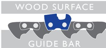
The Cutter **FALLS** back into place along the guide rail.
