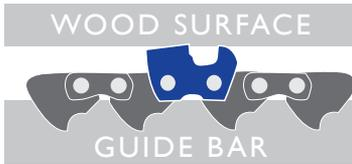
The Cutter's leading edge **CATCHES** the wood surface.
