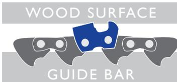
The depth gauge sinks into the wood and causes the Cutter to **RISE** off the guide bar.
